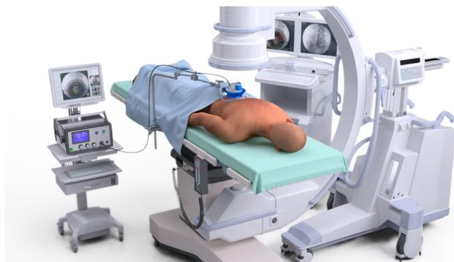
**Figure 2** The FUSMobile, Neurolyser XR, 1-MHz fluoroscopy-guided HIFU device. HIFU, high-intensity focused ultrasound.
