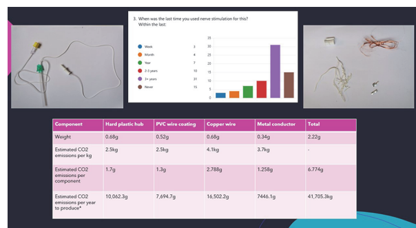
Abstract #35967 Figure 1 Last use of nerve stimulation graph, photos of needle equipment assembled and disassembled and box to demonstrate the environmental impact
