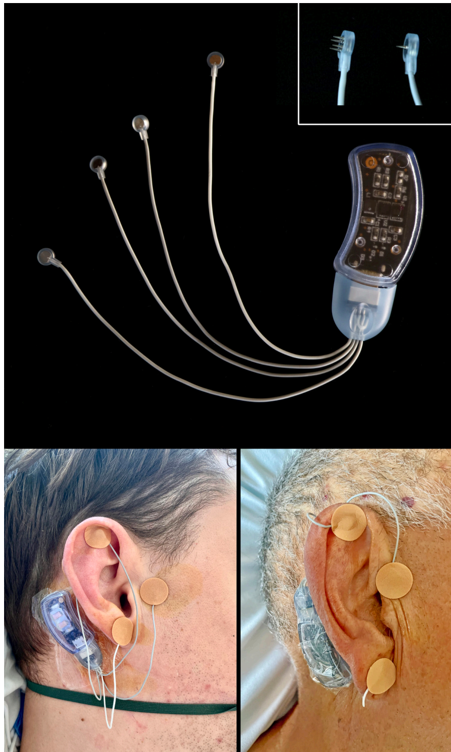
Figure 1 A percutaneous auricular nerve stimulation system (NSS-2 Bridge, Masimo, Irvine, California, USA). Each of the three electrodes has a 2-millimeter-long integrated needle/lead (inset) and the ground electrode has four 2-millimeter-long integrated needles/leads (inset). Used with permission from Brian M Ilfeld.
